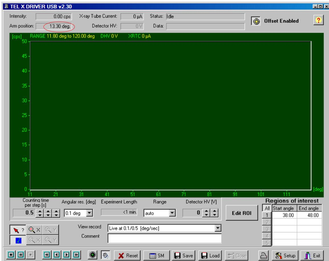
3. If the angle you noted in the previous step and the actual carriage arm position do not match, open the “Setup” window (button on lower right corner). In the “Arm Position” section, change the angle to reflect the actual position of the carriage arm and press “Set arm pos.”
